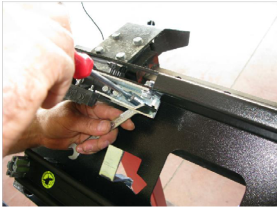
KİLİT GAGA YUVASI AYARI / SETTINGS OF LOCK BEAK SLOT
